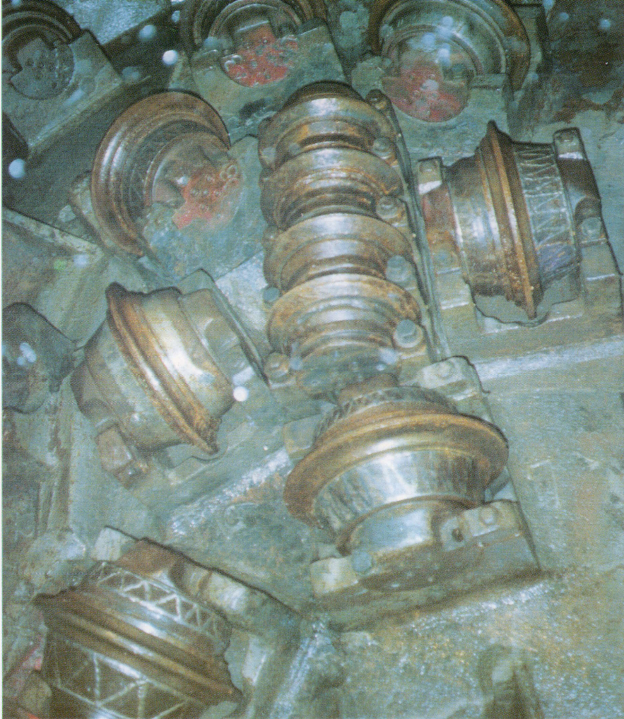
Cutterhead viewed from the relief drive.
